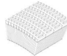
Lead tungstate crystals have a short radiation length (0.9cm) and Moliere radius (~ 2cm). This yields a high performance compact calorimeter with fine segmentation. The scintillation light is detected by specially developed Silicon Avalanche Photodiodes (APD) which allow an amplification of up to ~ 100
